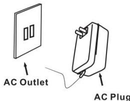
NOTE: You will note that this system is equipped with domestic standard AC power plug. If this plug does not fit into your existing AC outlet, do not try to defeat this safety feature by filing the wide blade to make it fit into your outlet. If this plug will not fit into your outlet, you probably have an outdated non-polarized AC outlet. You should have your outlet changed by a qualified licensed electrician.
