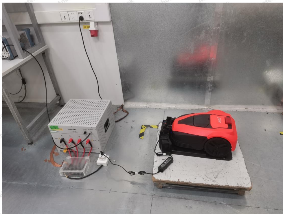
Photo of Conducted Emission Measurement
