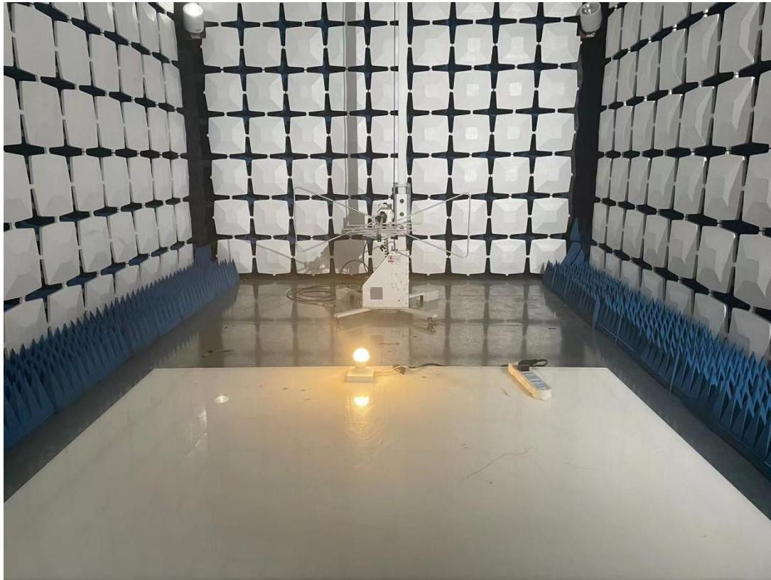
Below 1GHz for radiated emission test setup
