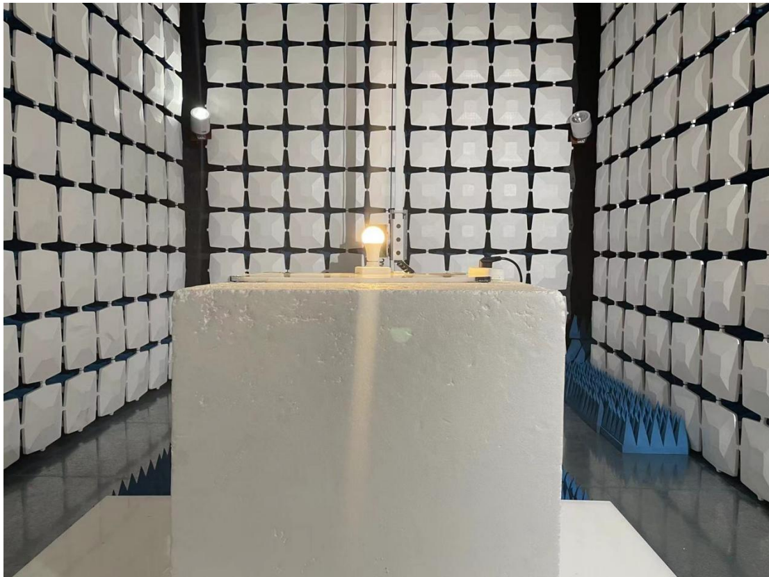
Above 1GHz for radiated emission test setup
