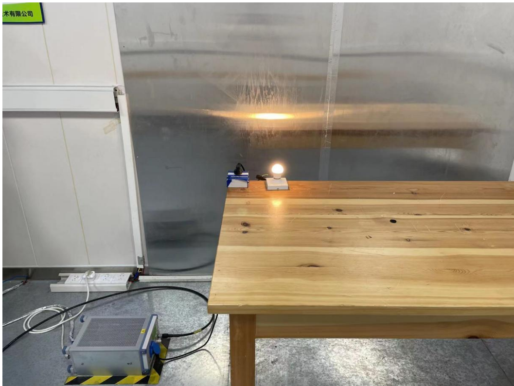
Conducted emission test setup
