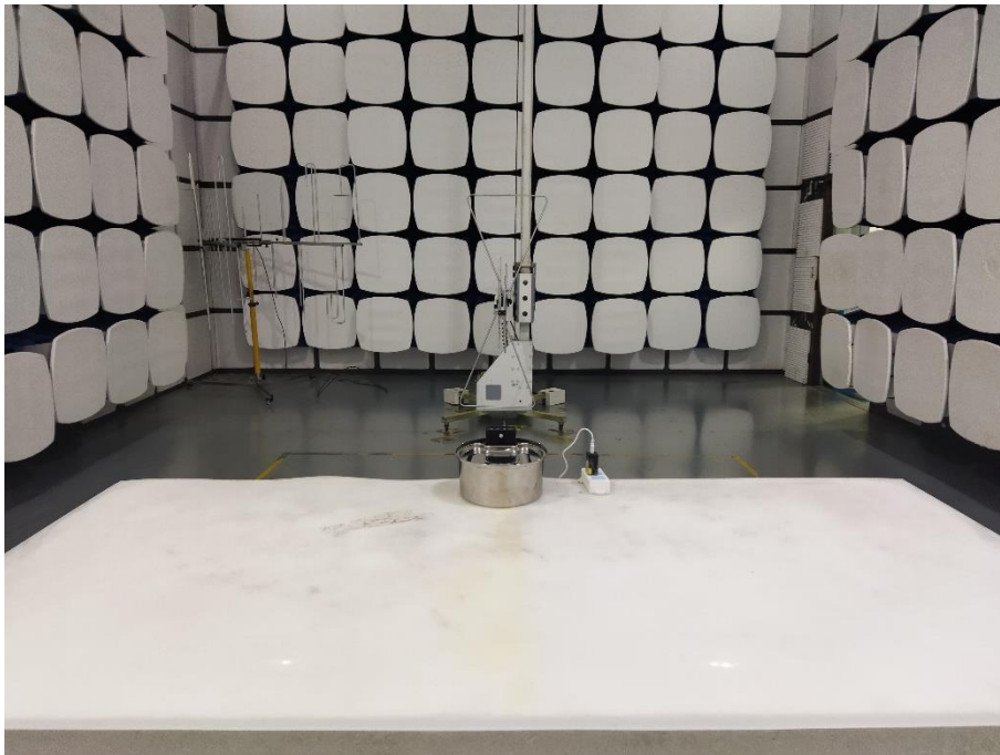
Photographs of the Test Set-up for Radiated Emissions(30-1000MHz)
