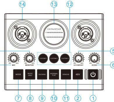
1. Power supply: Press the power key for three seconds to switch on, turn on the working indicator white.
