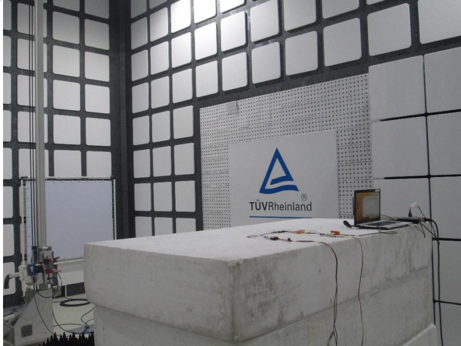
Photograph 5: Test Setup for Spurious Emissions (Back View 3)
