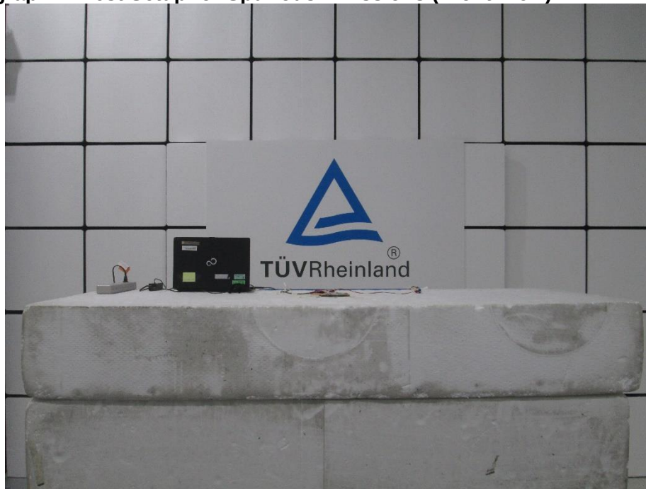
Photograph 8: Test Setup for Spurious Emissions (Back View 1)
