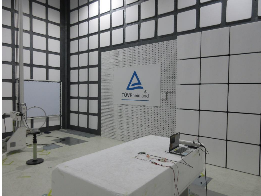
Photograph 3: Test Setup for Spurious Emissions (Back View 1)
