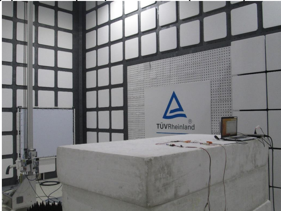
Photograph 6: Test Setup for Spurious Emissions (Back View 4)
