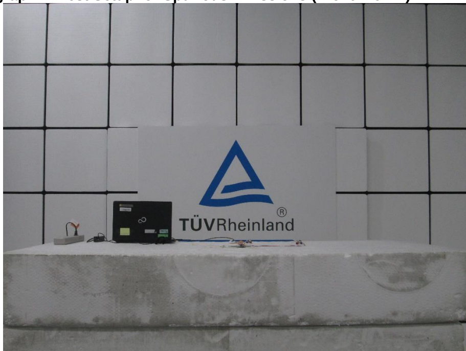
Photograph 2: Test Setup for Spurious Emissions (Front View 2)
