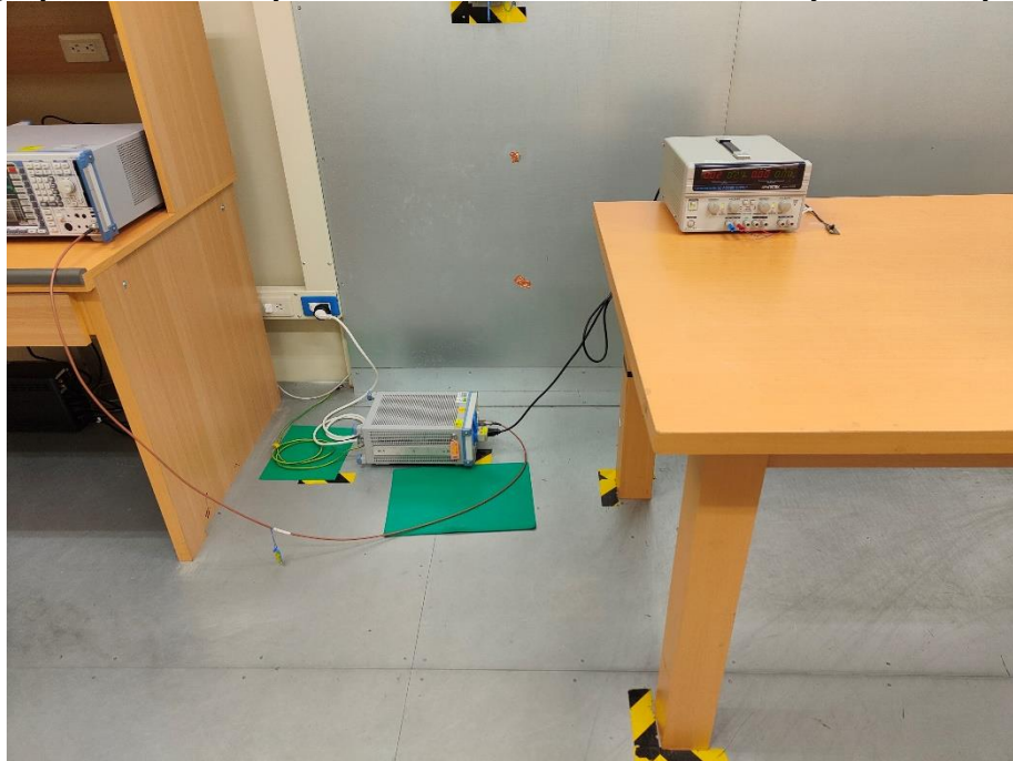
Photograph 8: Test Setup for Mains Conducted Emissions (Front View)
