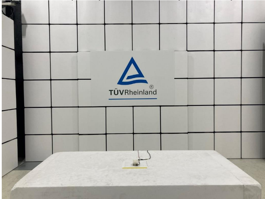
Photograph 1: Test Setup for Spurious Emissions (Front View 1)
