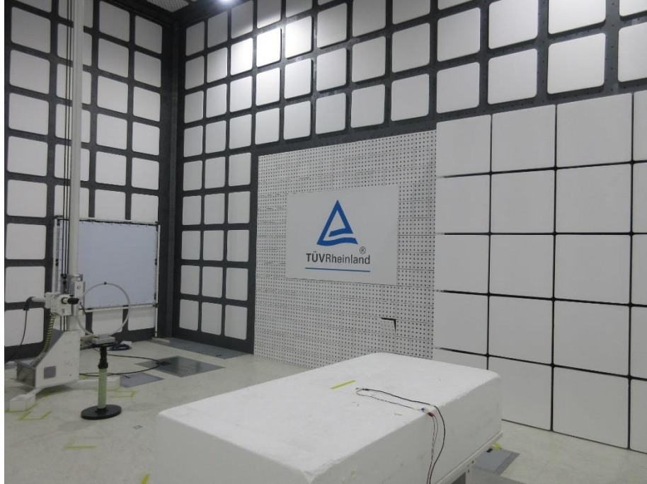
Photograph 3: Test Setup for Spurious Emissions (Back View 1)
