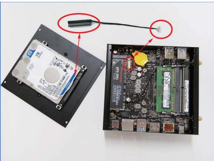
11. Connect the hard drive and motherboard with an accessory cable.
