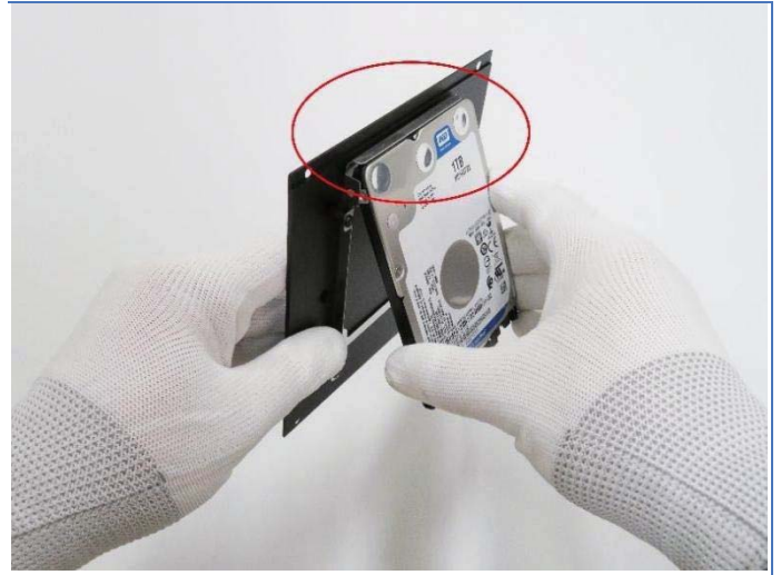
8. Align the hard drive with the bracket.
