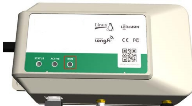
Figure 6: Observe the RUN Indicator
