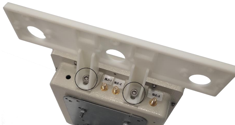
Figure 11: Fitting room antenna mount
