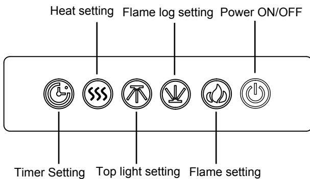
You can keep pressing "Flame setting" button for 10 seconds to connect to the mobile APP.
