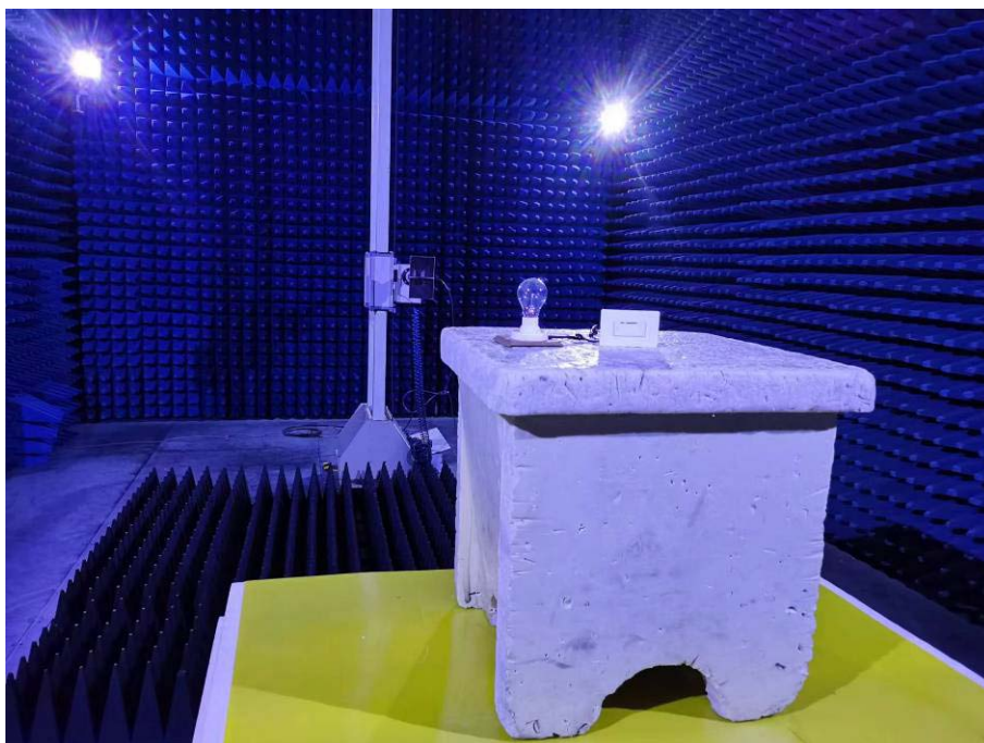
Photo of Radiated Emission Measurement (Above 1G)
