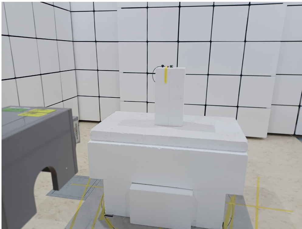
Radiated Test (Horn) (40GHz-50GHz)
