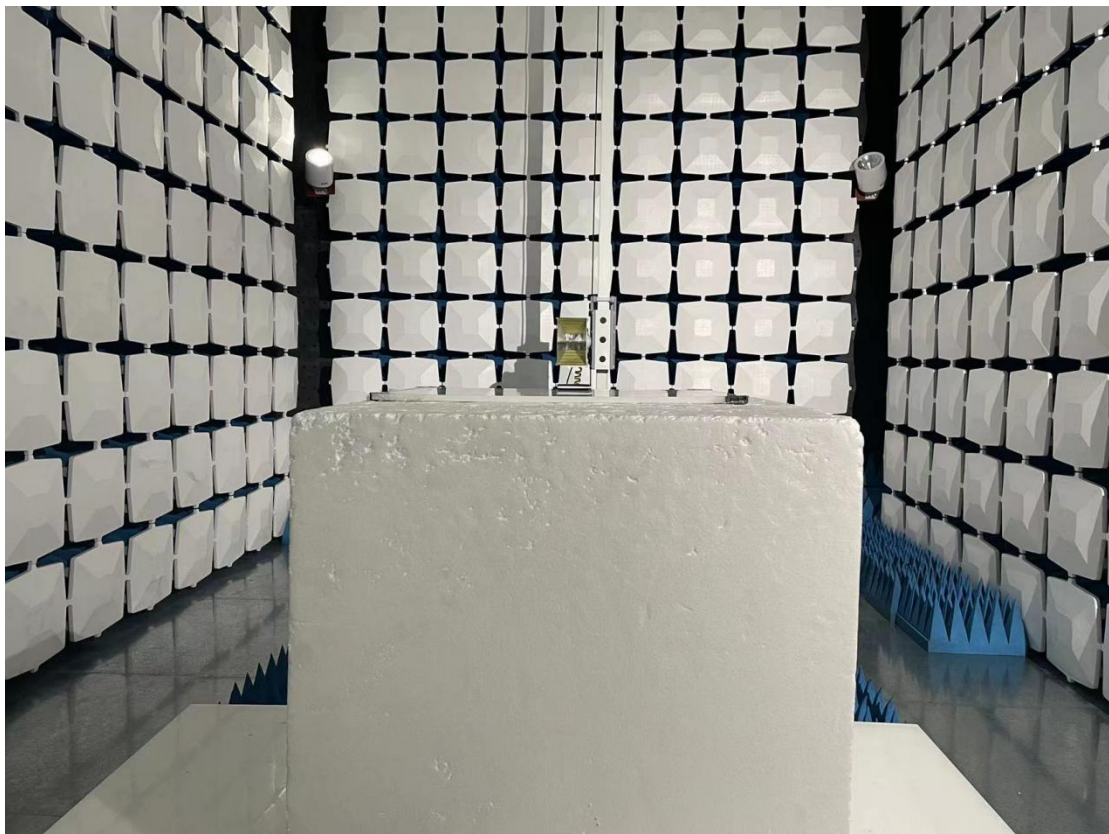
Above 1GHz for radiated emission test setup
