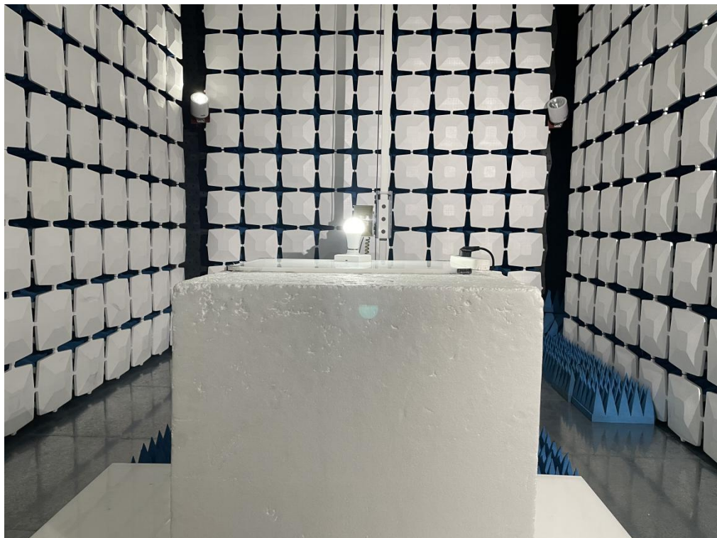
Above 1GHz for radiated emission test setup
