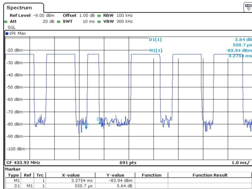
The graph shows the duration of 'on' signal. From Marker 1 to Delta 2, duration is 0.551ms.
