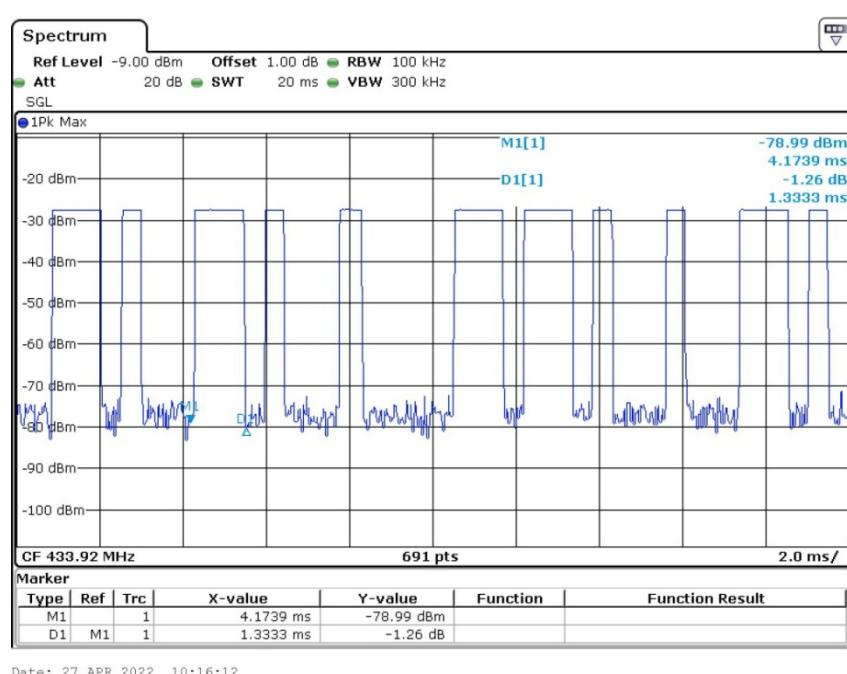
The graph shows the duration of 'on' signal. From Marker 1 to Delta 2, duration is 1.333ms.
