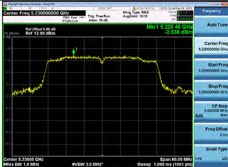
Power Spectral Density NVNT_ANT1_802_11n(HT40)_5230_40M
