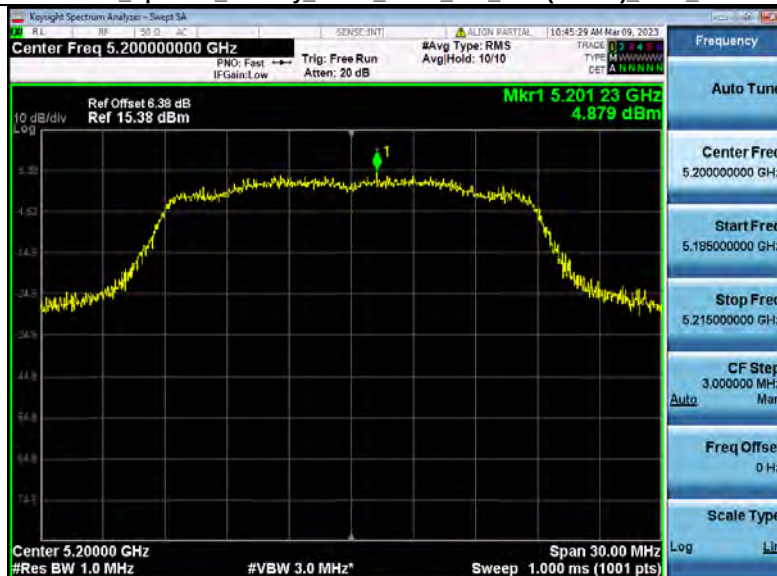
Power Spectral Density NVNT_ANT1_802_11ac(VHT20)_5200_20M
