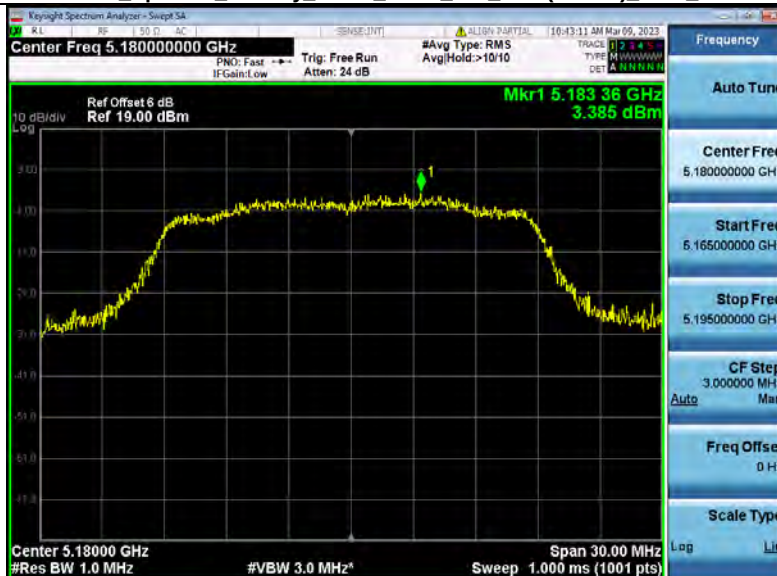
Power Spectral Density NVNT_ANT1_802_11ac(VHT20)_5180_20M
