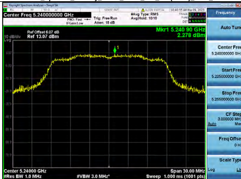
Power Spectral Density NVNT_ANT1_802_11n(HT20)_5240_20M
