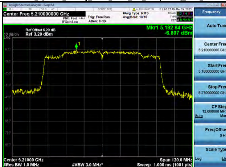
Power Spectral Density_NVNT_ANT1_802_11ac(VHT80)_5210_80M
