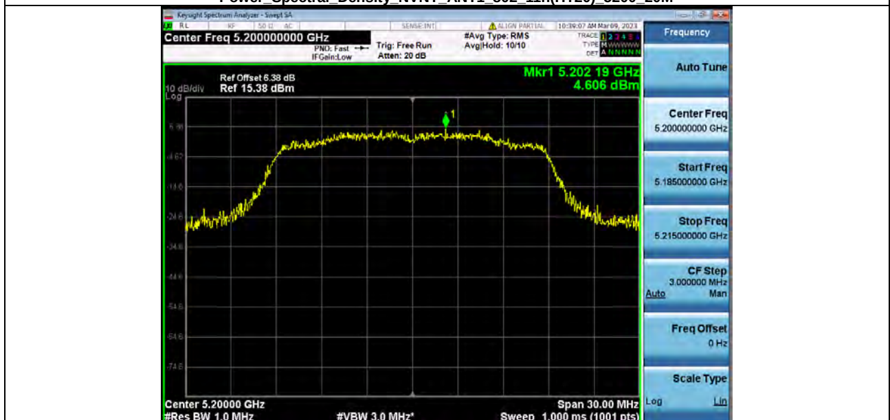
Power Spectral Density NVNT ANT1 802_11n(HT20) 5200_20M
