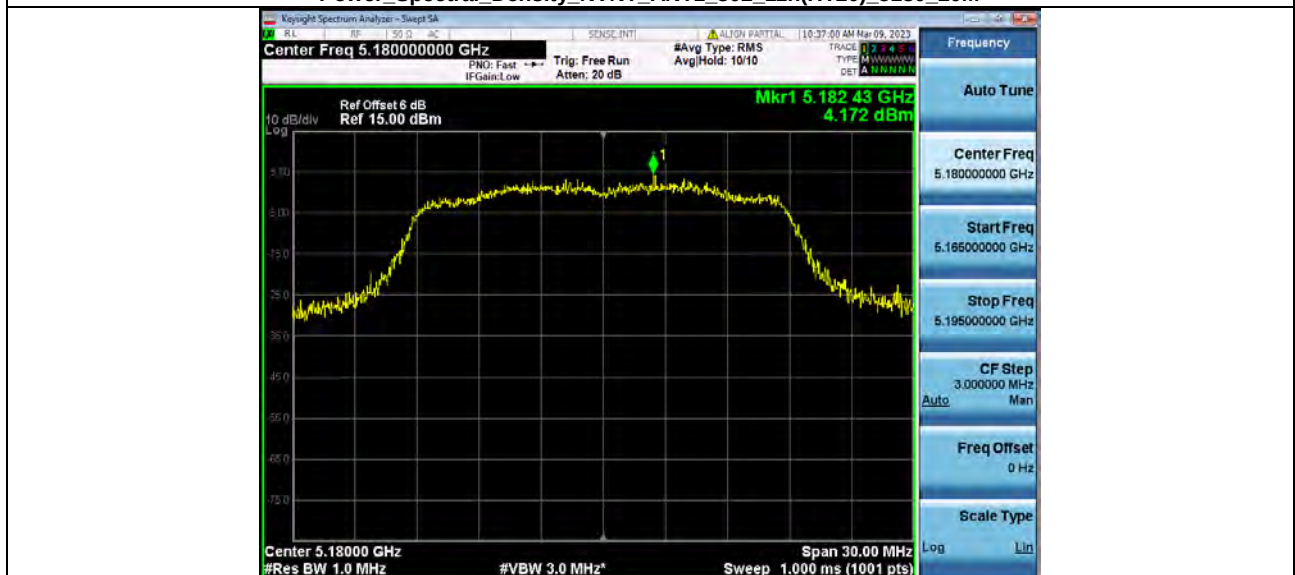
Power Spectral Density NVNT ANT1 802_11n(HT20) 5180_20M
