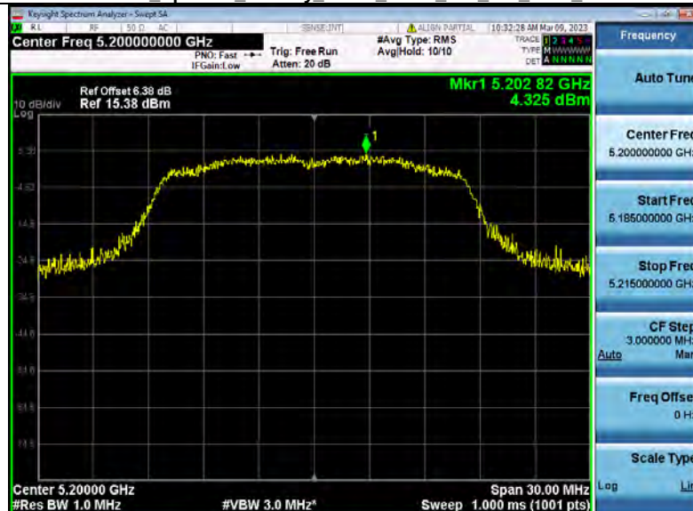
Power Spectral Density NVNT ANT1 802_11a 5200_20M
