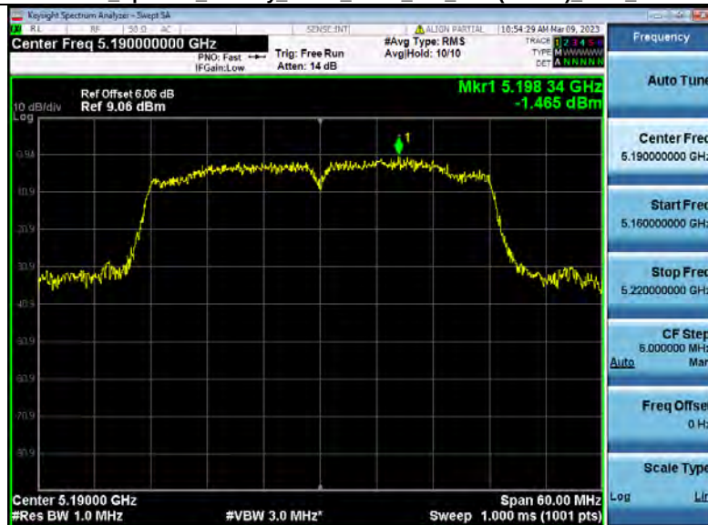
Power Spectral Density_NVNT_ANT1_802_11ac(VHT40)_5190_40M
