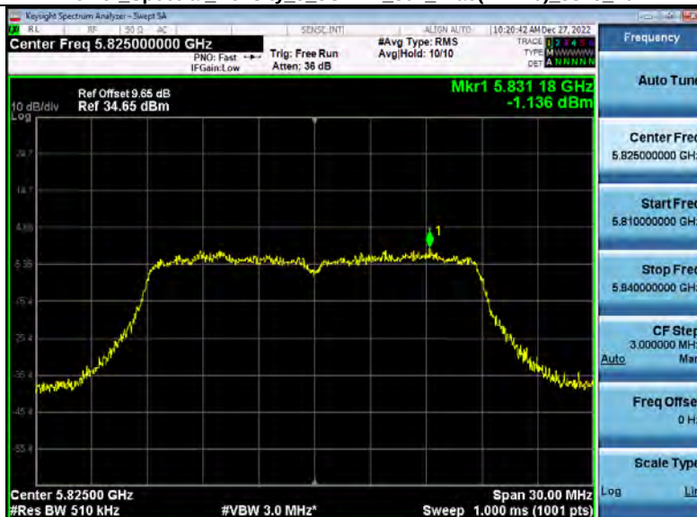
Power Spectral Density 5_8WiFi 802_11ac(VHT20)_5825_20M
