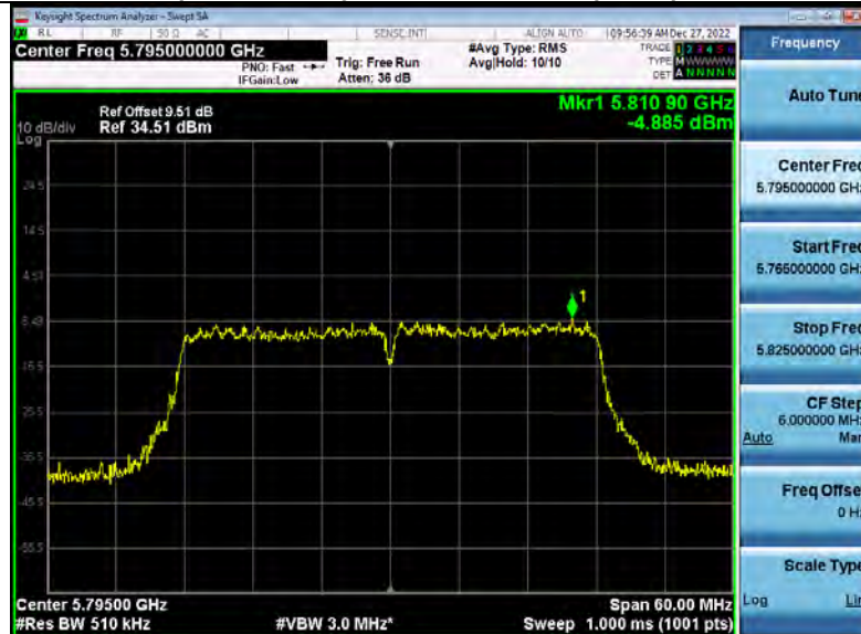
Power Spectral Density 5_8WiFi 802_11ac(VHT40) 5795_40M
