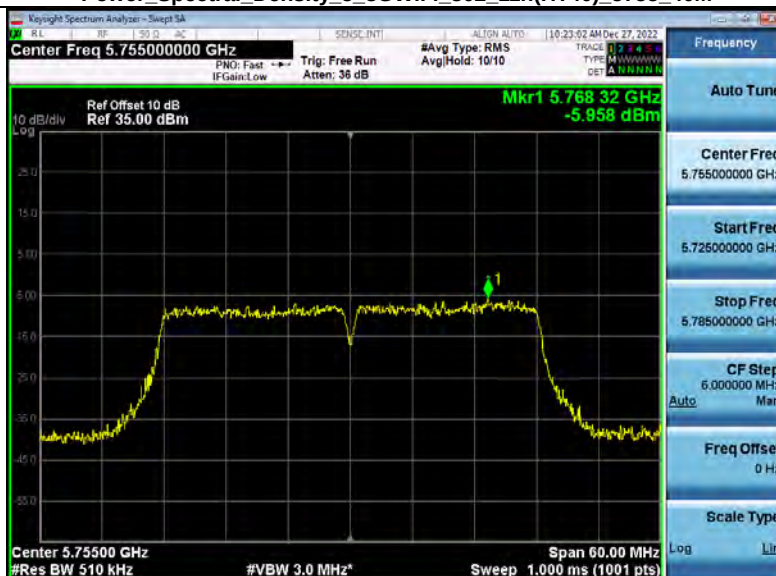
Power Spectral Density 5_8WiFi 802_11n(HT40)_5755_40M
