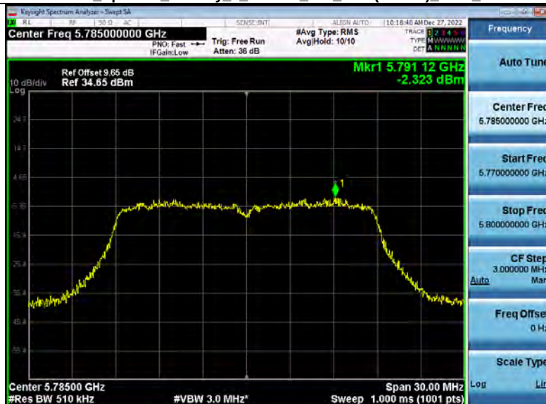
Power Spectral Density 5_8WiFi 802_11ac(VHT20)_5785_20M
