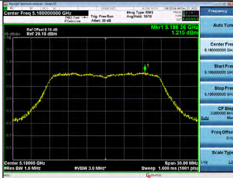
Power Spectral Density 5 2GWiFi 802 11ac(VHT20) 5180 20M
