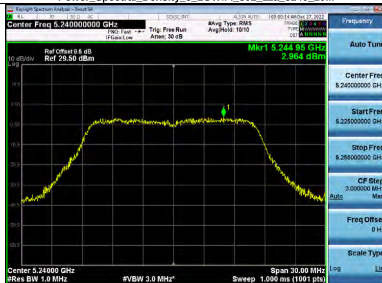
Power Spectral Density 5_2GWiFi_802_11a_5240_20M
