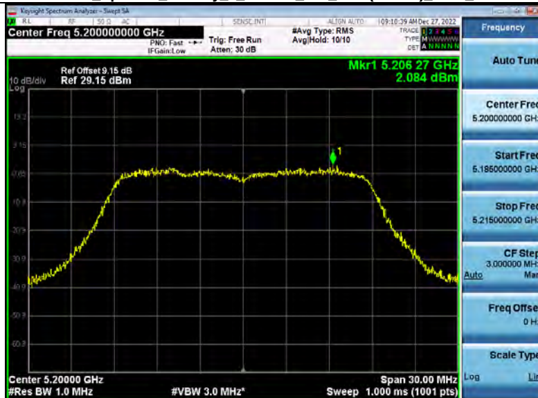
Power Spectral Density 5_2GWiFi_802_11ac(VHT20)_5200_20M
