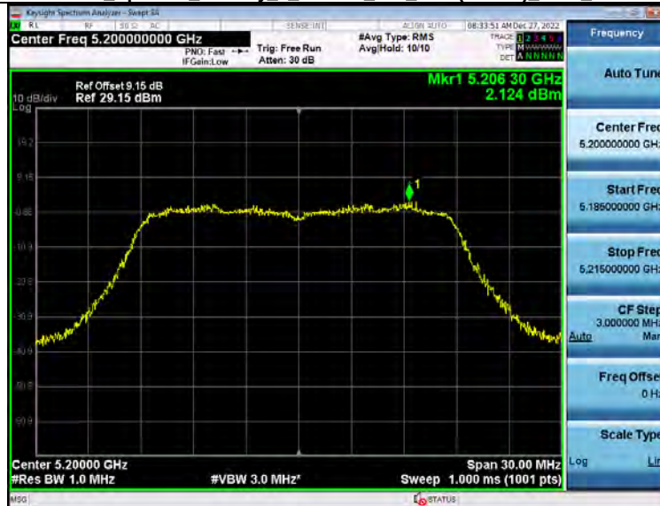
Power Spectral Density 5 2GWiFi 802 11ac(VHT20) 5200 20M
