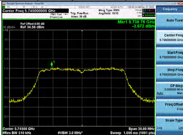
Power Spectral Density 5_8WiFi_802_11ac(VHT20)_5745_20M
