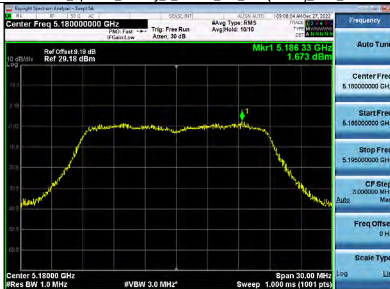
Power Spectral Density 5_2GWiFi_802_11ac(VHT20)_5180_20M
