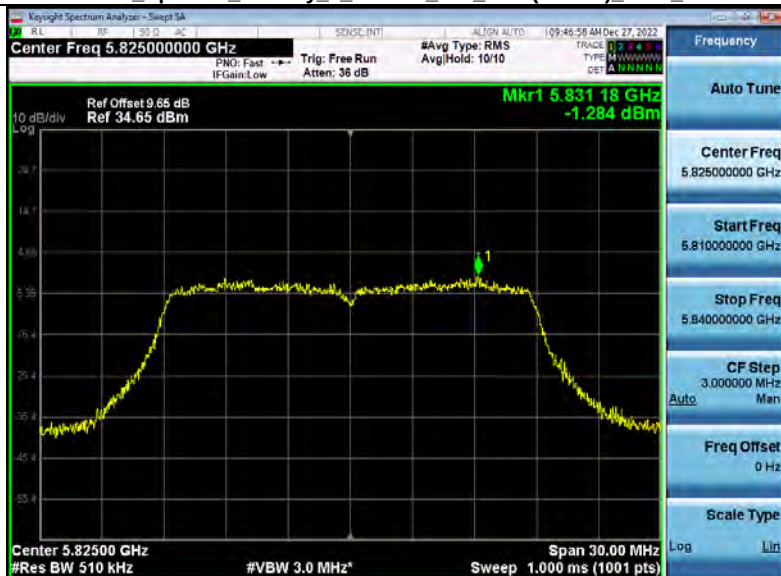
Power Spectral Density 5_8WiFi_802_11ac(VHT20)_5825_20M
