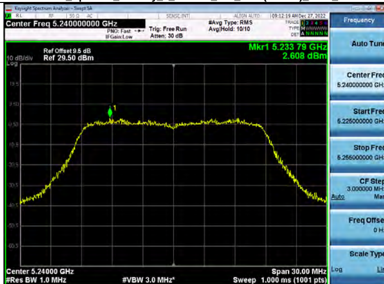
Power Spectral Density 5_2GWiFi_802_11ac(VHT20)_5240_20M
