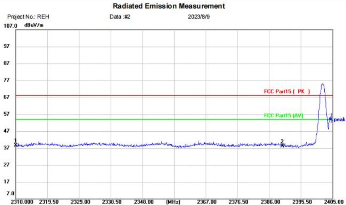
Site: Polarization: **Vertical** Temperature: (C)
