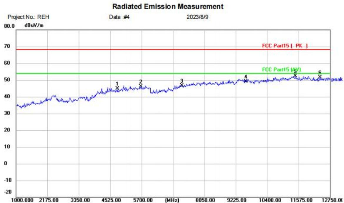
Site: Limit: FCC Part15 ( PK ) EUT: Portable Record Player M/N: PT-02 Mode: TX-L Note: Polarization: **Vertical** Power: Temperature: (C) Humidity: %RH
