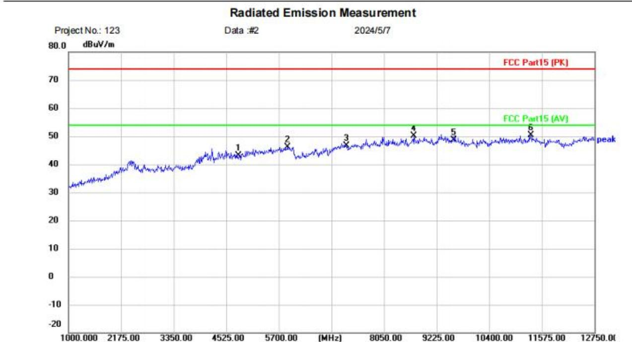
Site: Limit: FCC Part15 (PK) EUT: ALL IN ONE RECORD PLAYER M/N: TR-19PCD Mode: TX-2402 Note: Polarization: **Vertical** Power: Temperature: (C) Humidity: %RH
