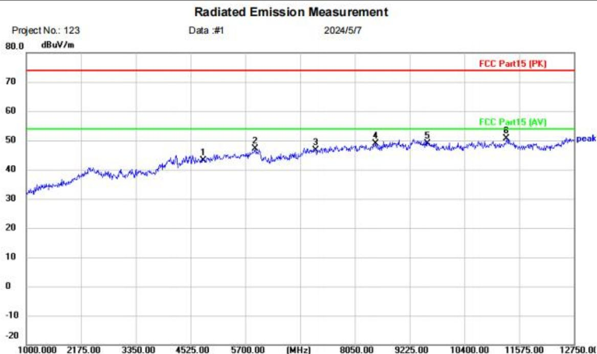
Site: Polarization: **Horizontal** Temperature: (C)
