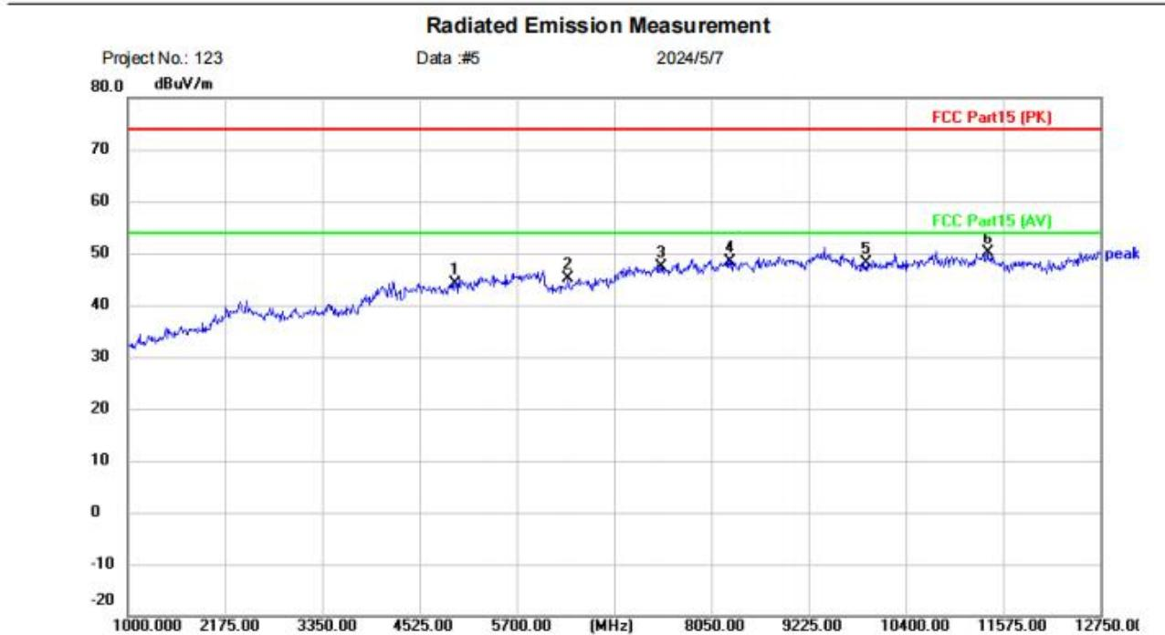
Site: Limit: FCC Part15 (PK) EUT: ALL IN ONE RECORD PLAYER M/N: TR-19PCD Mode: TX-2480 Note: Polarization: **Horizontal** Power: Temperature: (C) Humidity: %RH
