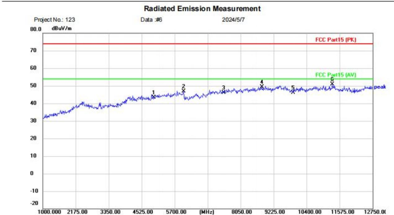
Site: Limit: FCC Part15 (PK) EUT: ALL IN ONE RECORD PLAYER M/N: TR-19PCD Mode: TX-2480 Note: Polarization: **Vertical** Power: Temperature: (C) Humidity: %RH
