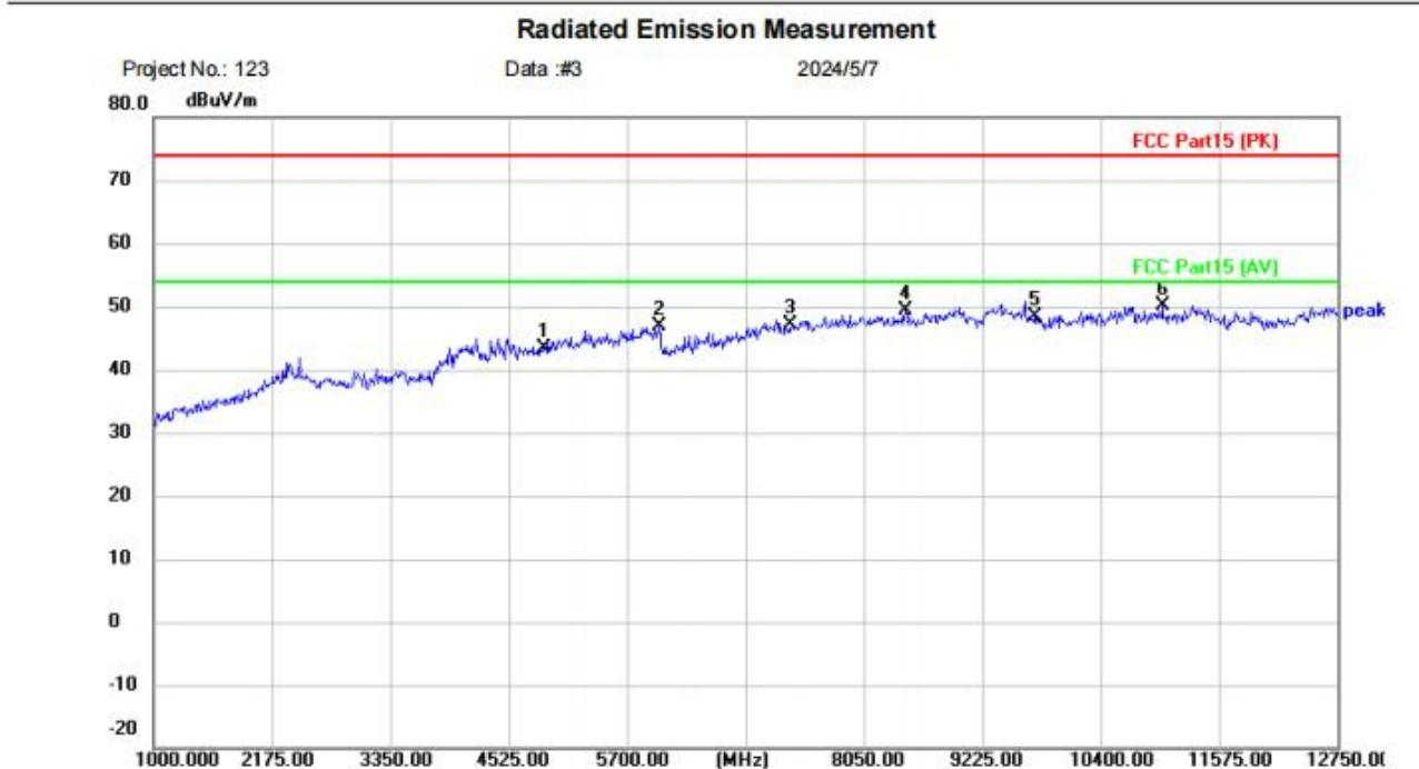
Site: Limit: FCC Part15 (PK) EUT: ALL IN ONE RECORD PLAYER M/N: TR-19PCD Mode: TX-2441 Note: Polarization: **Vertical** Power: Temperature: (C) Humidity: %RH
