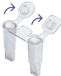
4. Tilt the sample tube to 45 degrees, and gently squeeze it to let 2 drops of solution each fall into the 2 openings of the test tube. Then, close the cap of the test tube.
