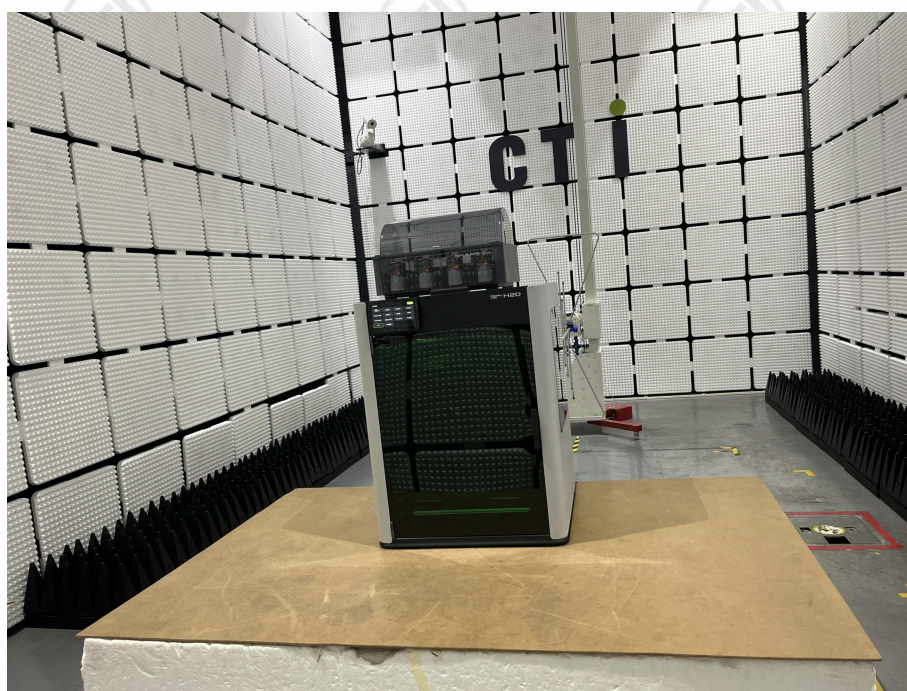
Radiated Spurious Emissions Test Setup (30MHz ~ 1GHz)
