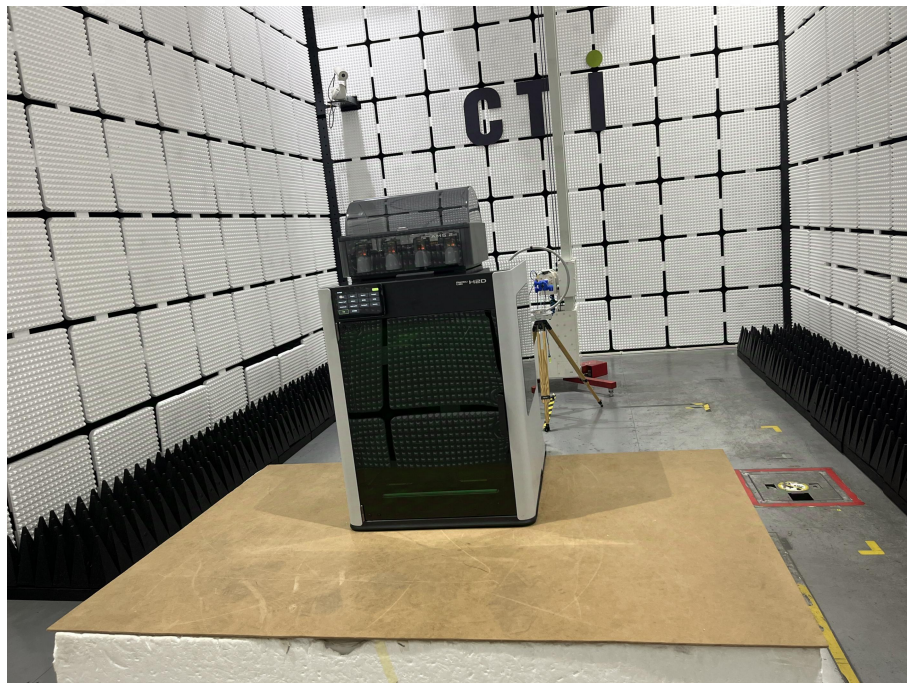
Radiated Spurious Emissions Test Setup (9kHz ~ 30MHz)
