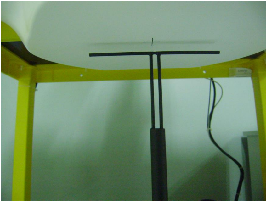
Setup Photo of Dipole Antenna
