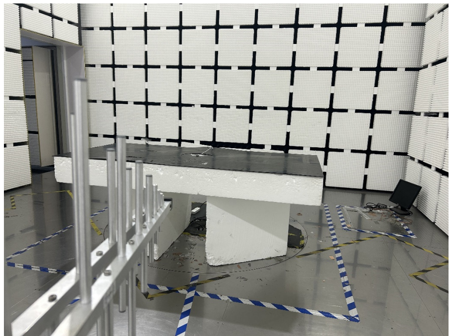
Radiation Emission Test Setup (30MHz to 1GHz)
