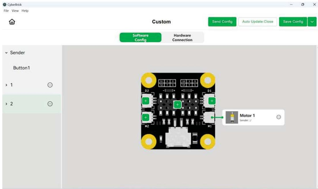
Adjust the maximum speed and bias for forward and reverse motor rotation in the Modify interface. The Haptic Optimization allows the relationship between the joystick value and the motor speed to become non-linearly proportional (not a first-order linear relationship), so that the low-speed control is more accurate and the high-speed response is faster. You can specifically adjust the effect of haptic optimization in Edit.
