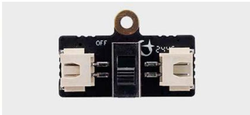
Power switch module is a two-position switch that is often used to control power on/off without removing the battery.
