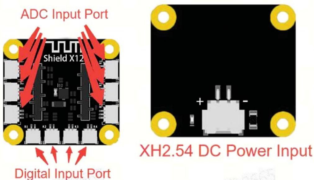
On the left and right sides of the transmitter shield, there are respectively 3 ADC input channels. Below it, there are 4 digital input channels. The gray slot on the back is the slot for the multi-function controller core. It can be powered through the XH2.54
