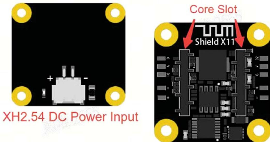
On the left and right sides of the receiver shield, there is respectively a DC motor port and a WS2812 port. In the center, there are 4 servo ports. It can be powered through the XH2.54 power input.
