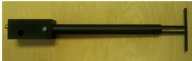
Figure 1 – MVG COMOSAR Validation Dipole
