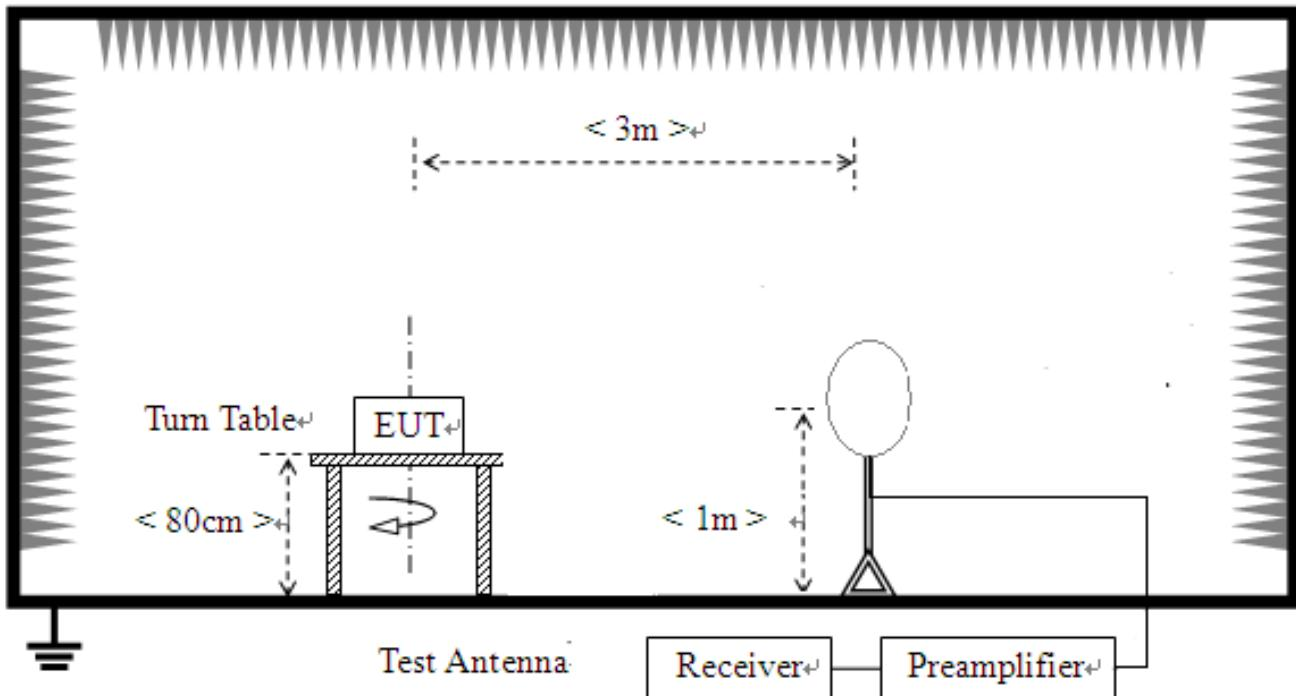
For radiated emissions from 30MHz to 1GHz
