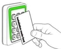
Resetting the OSDP secure channel.
