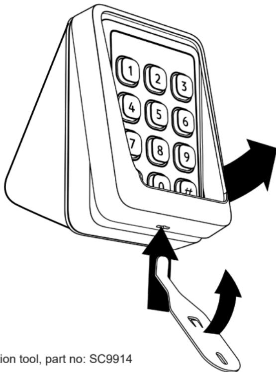
Cidron installation tool, part no: SC9914
