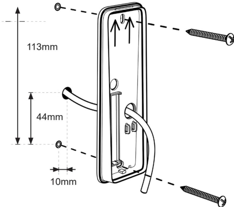
When installing directly to wall or door, use the installation holes as picture describes. If using other screws than the ones supplied with the reader, make sure to use a flat headed screw with a maximum height of 2.8 mm and a maximum diameter of 7.8 mm on the screw head.
