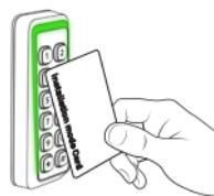
Resetting the OSDP secure channel.
