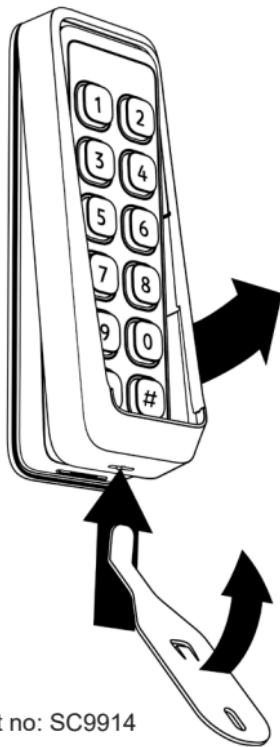
Cidron installation tool, part no: SC9914
