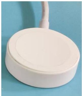
Connect the cable to the Micro USB socket, and place the smart watch on the wireless charger. If the watch is on, it indicates that the charging is in progress. At the same time, you can check the battery charge status on the smart watch screen.
