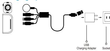
1: Connect the USB-A or TYPE-C interface to the power adapter.
