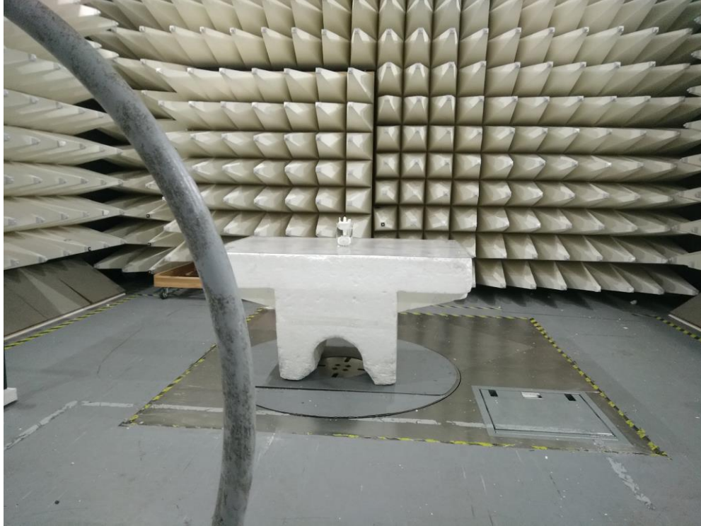
Photograph No.7 SAC Setup for carrier field strength measurements below 30 MHz, 3 m distance for 8MHz
