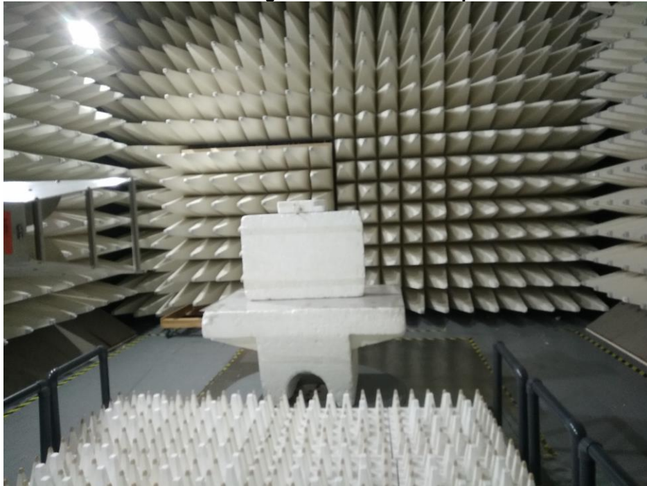
Photograph No.3 Carrier field strength measurement setup for BLE
