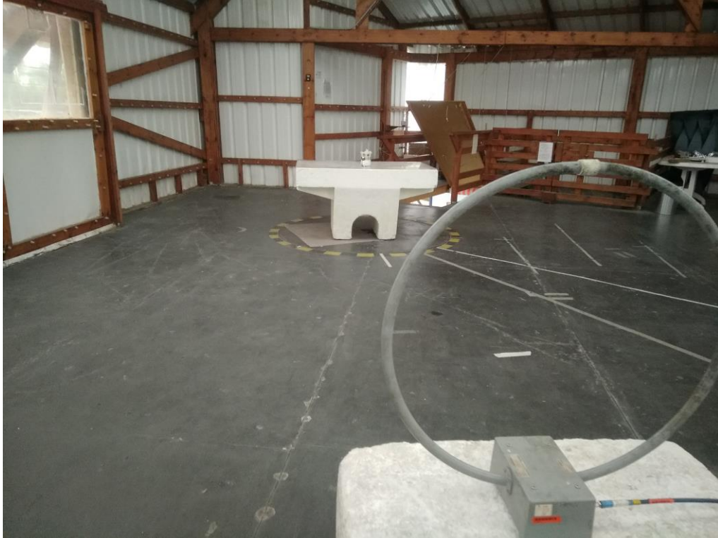
Photograph No.5 OATS Setup for carrier field strength measurements below 30 MHz, 5 m distance for 8MHz
