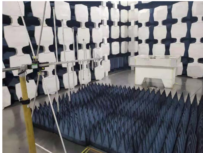
(2) Radiated spurious emission Test Setup (Below 1 GHz)
