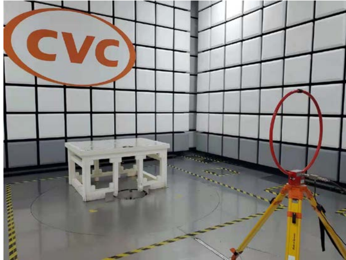
(1) Radiated spurious emission Test Setup(Below 30MHz)
