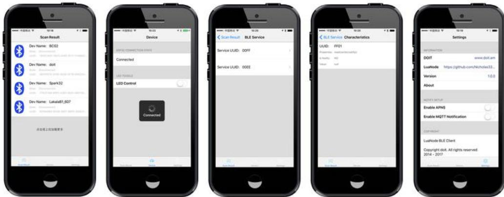
To control the LED on ESP32 board, you have to build the example `esp32_ble_gatt_server_led_control_for_phone`, and then download the firmware. Run the `LuaNode_BLE_Client` and then toggle the LED switch on app to turn on/off the LED on board. The following video is a test for ESP32: <https://www.youtube.com/watch?v=LhvA33yf7P8>
