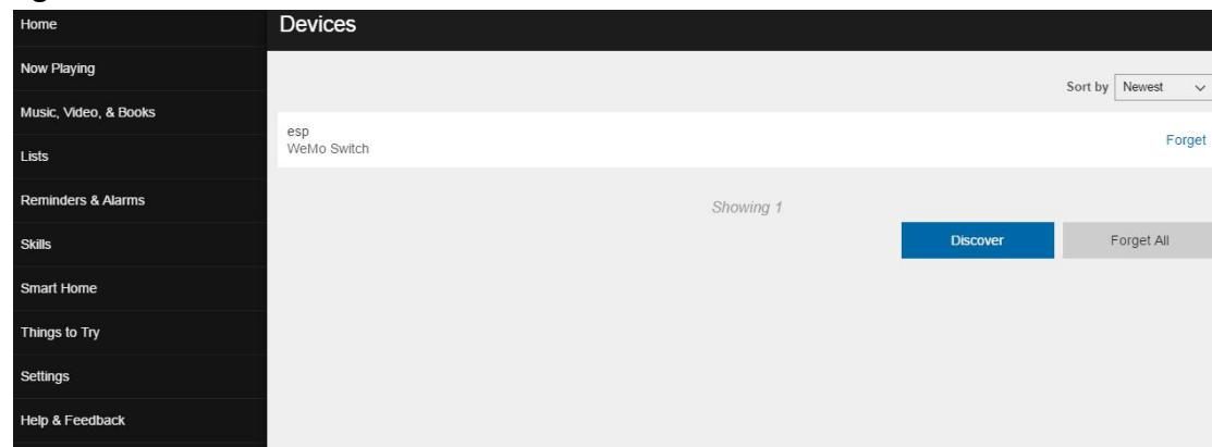
When Alexa find ESP32 device successfully, you can ask Echo Dot "Alexa, turn on ESP" to turn on the blue LED on ESP32 board. Ask "Alexa, turn off ESP" to turn off the LED. The following link is a video to show the ESP32 voice control via Amazon Echo Dot: <https://youtu.be/Eg1dApUHIBc>
