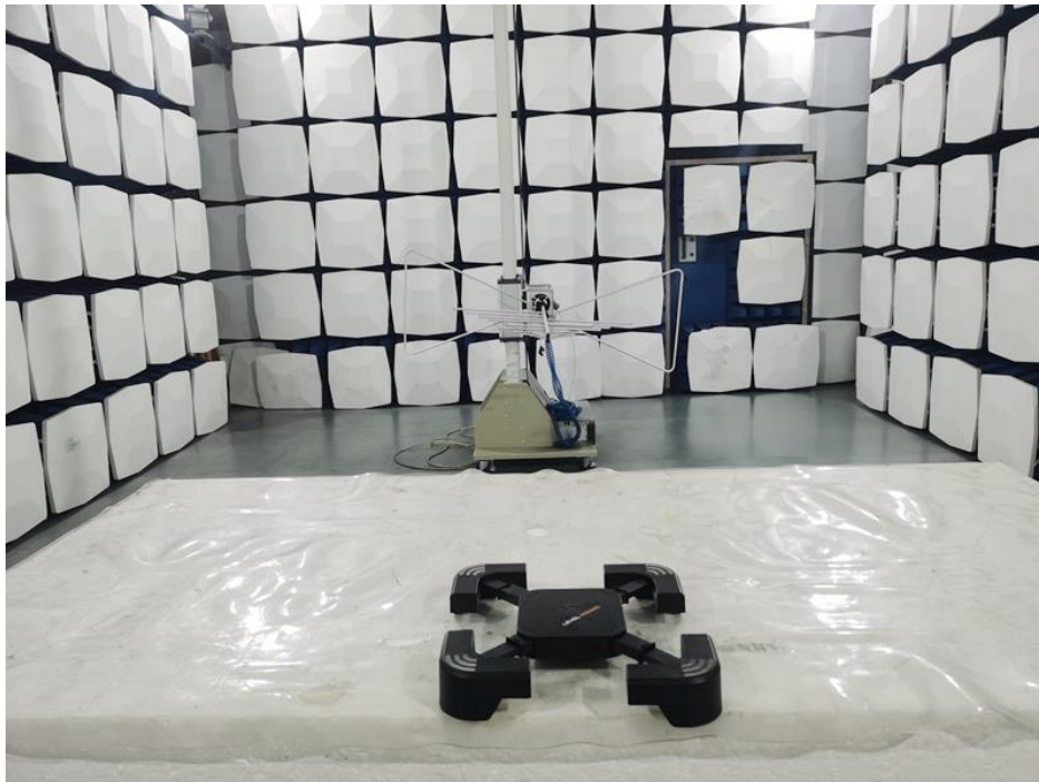
Radiated Emission Test Setup:
