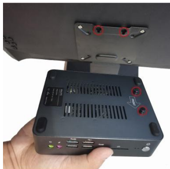
5. Attach the PC to the screw hole of the bracket
