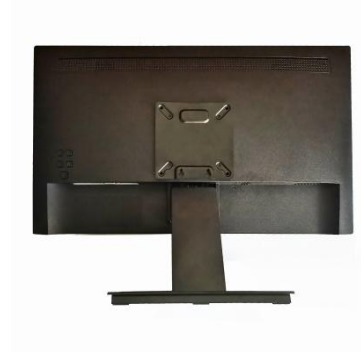
2. Put the vesa to 4 screws holes
