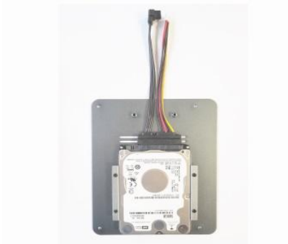
5.Put the HDD on the Button cover and connect Cable
