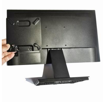
1. Attach mount vesa to the back of the display
