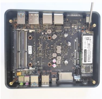
3.Locking the screw of SSD
