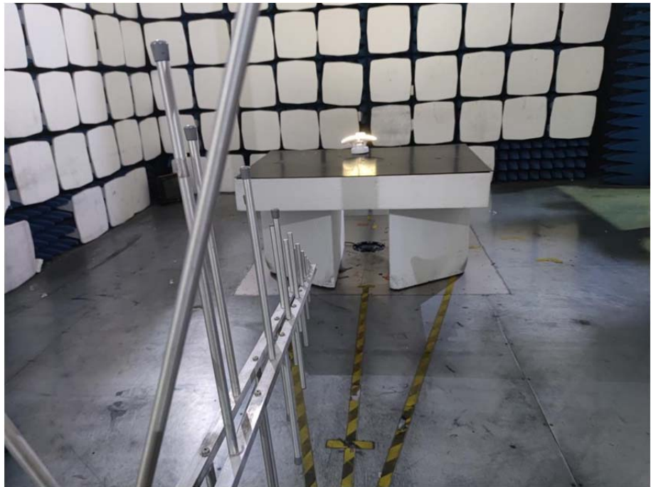
Radiation Emission Test Setup (30MHz to 1GHz)
