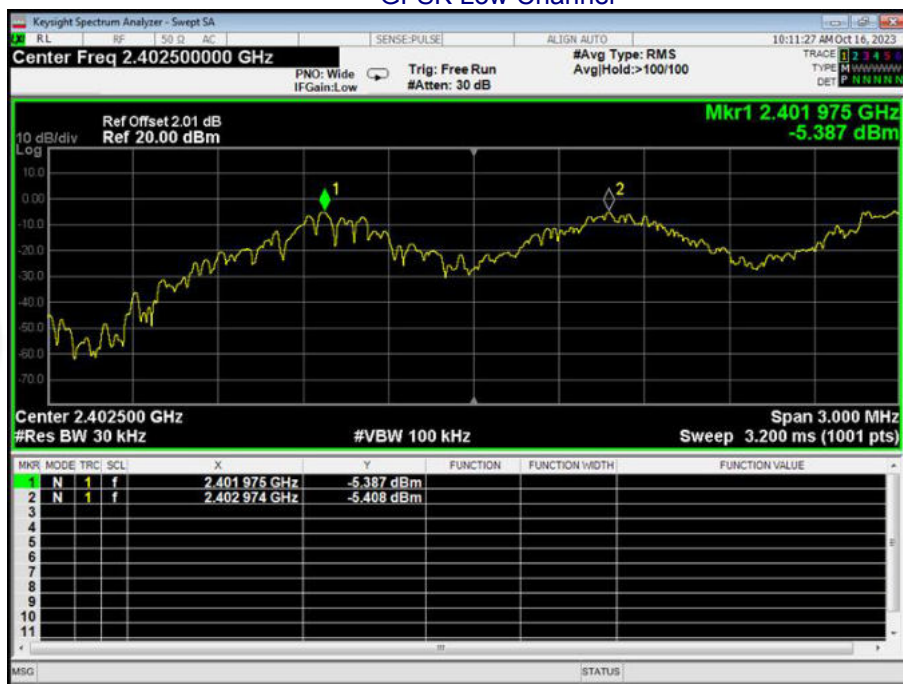
Test plots GFSK Low Channel
