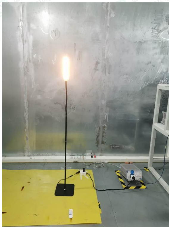
Test Setup Photo of Line Conducted Emissions Measurement
