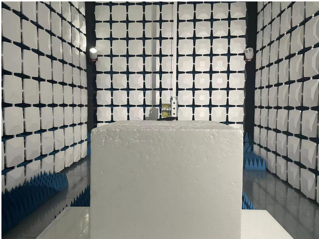
Above 1GHz for radiated emission test setup
