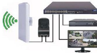
The CPE connects to the POE port of the POE power adapter, the LAN port of the POE power adapter connects to switch or video recorder.
