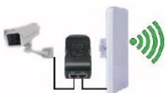
The CPE connects to the POE port of the POE power adapter, the LAN port of the POE power adapter connects to the IP camera.
