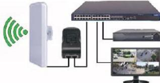
The CPE connects to the POE port of the POE power adapter, the LAN port of the POE power adapter connects to switch or video recorder.
