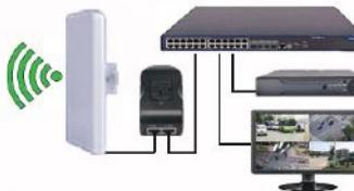
The IP cameras all connect to the switch, the LAN port of the POE power adapter connects to the switch, and POE port of the POE power adapter connects to the CPE.
