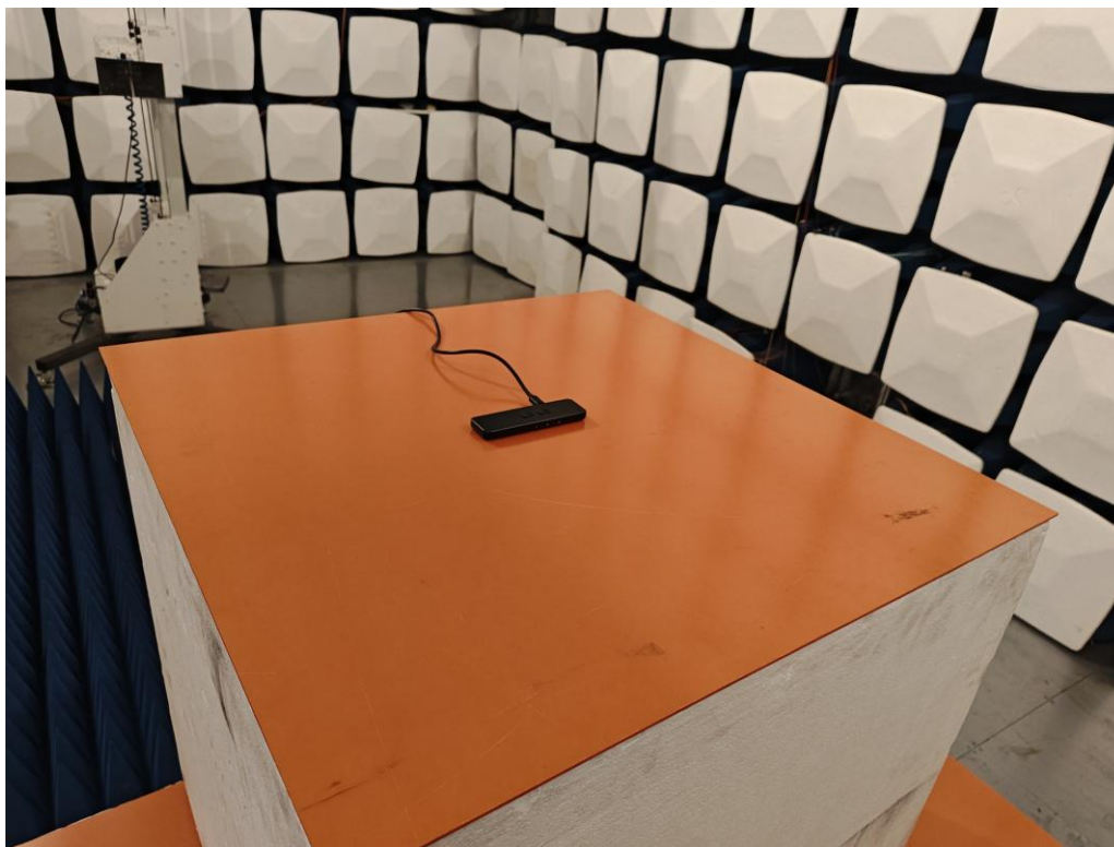
Fig. 3 Test Setup Photo(s) of Conducted Emissions Measurement
