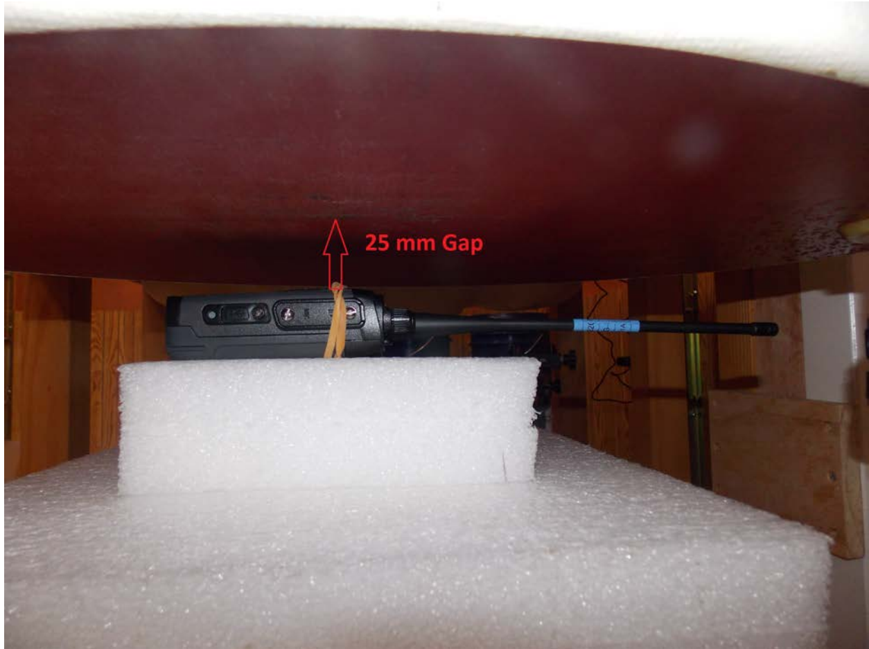
Face Test Position with 25 mm Gap
