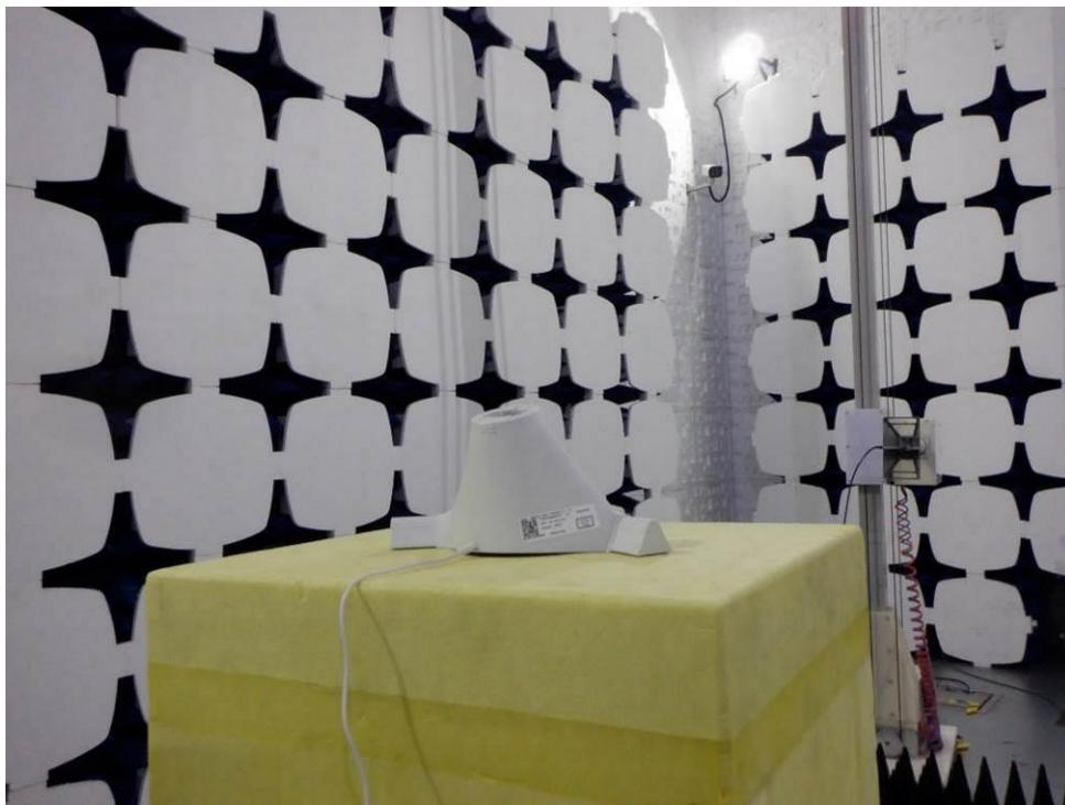
**Radiated Spurious Emissions Below 1GHz**
