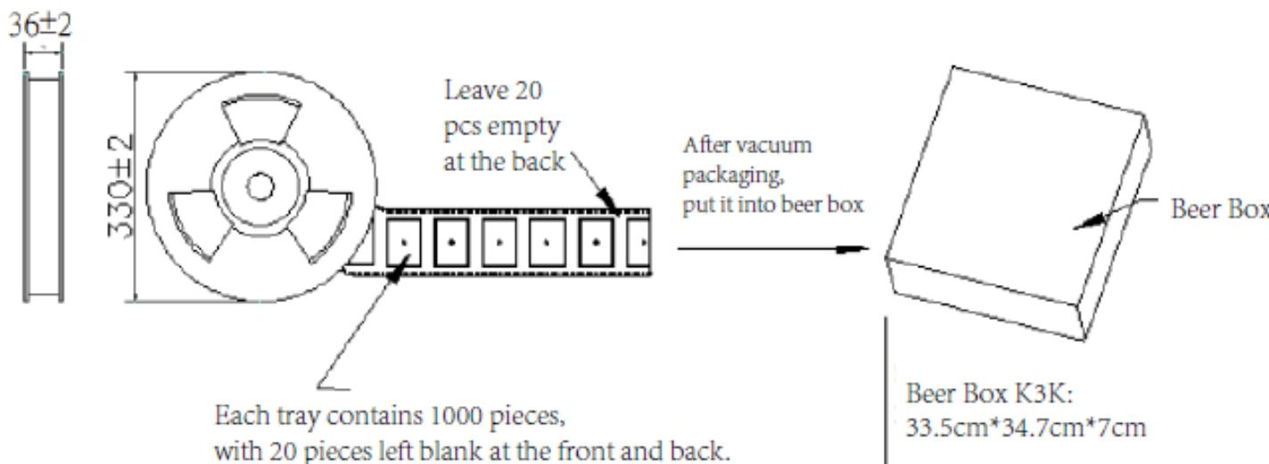
1. Each reel of tape contains 1000 units (20 compartments are left empty at the front and back for unused products).
