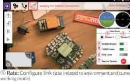
① Rate: Configure link rate (related to environment and current working mode).
