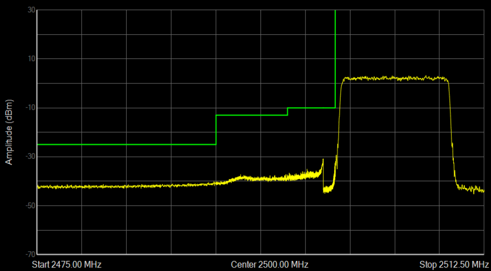
Band7 QPSK BW=10MHz Channel=20800 RB Size=50 Position=#0
