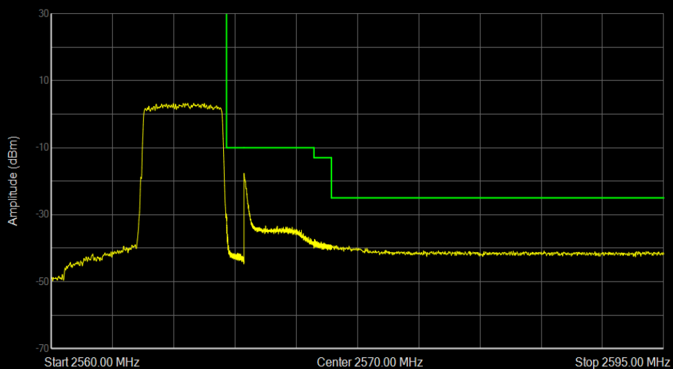
Band7 QPSK BW=5MHz Channel=21425 RB Size=25 Position=#0
