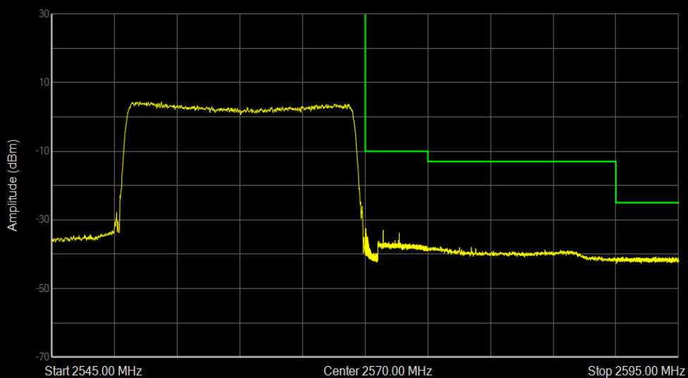
Band7 QPSK BW=20MHz Channel=21350 RB Size=100 Position=#0
