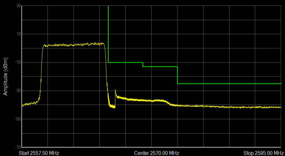
Band7 QPSK BW=10MHz Channel=21400 RB Size=50 Position=#0
