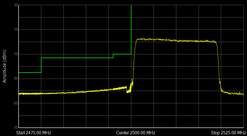
Band7 QAM16 BW=20MHz Channel=20850 RB Size=100 Position=#0
