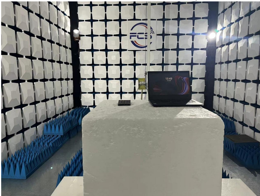
Above 1GHz for radiated emission test setup
