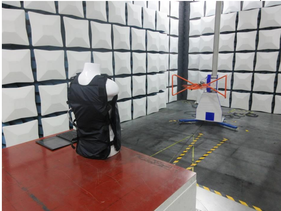
RADIATED RF MEASUREMENT SETUP (30MHz ~ 1 GHz)
