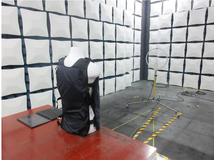
RADIATED RF MEASUREMENT SETUP (9KHz ~ 30 MHz)
